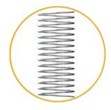
0.4 ohm (rated at 25-30 watts) Φ0.5mm Spacing:1mm
